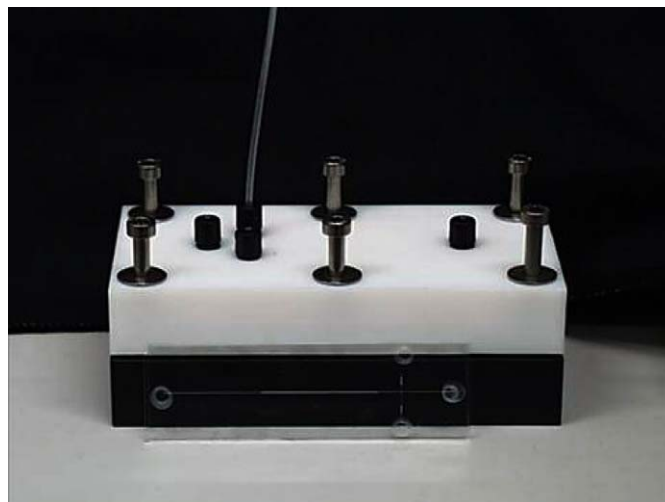
Fig. 6. High pressure microchip connection module for the microchips with reservoirs.
